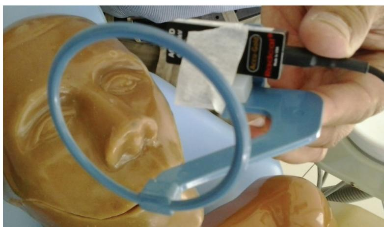
**Figure 1** – Head and neck prototype containing real bones and equivalent tissue
