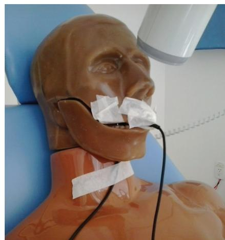
**Figure 3** – Head and neck prototype with sensor and ionization chamber in the sublingual gland
