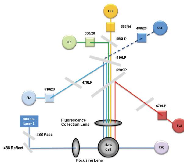
Subtitle – A laser beam excites the fluorochrome whose light is scattered frontally (FSC) and sideways (SSC). Argon laser is directed laterally by a mirror 488Pas and 488Reflect. Filter 530/28 BP capture the emission of FL1 and filter 555LP reflects the emission of FL1 and
